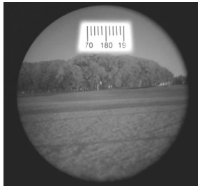
FIGURE 2-13. VIEW THROUGH INSTALLED COMPASS
