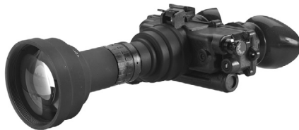
FIGURE 2-10. PVS-7 WITH MAGNIFIER LENS ASSEMBLY INSTALLED
