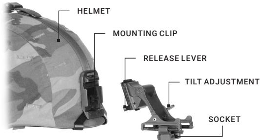
FIGURE 2-9. QUICK DISCONNECT HELMET MOUNT FEATURES
