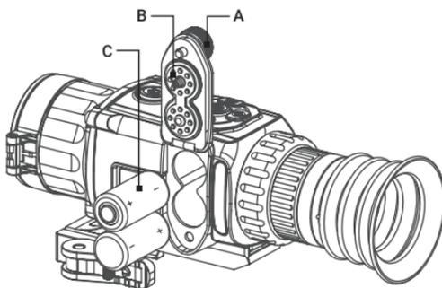
FIGURE 2-1. BATTERY INSTALLATION
