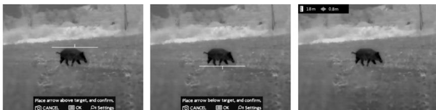
FIGURE 2-11. DISTANCE MEASUREMENT
