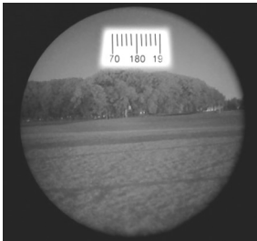
FIGURE 2-13. VIEW THROUGH INSTALLED COMPASS
