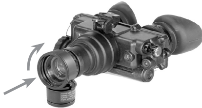
FIGURE 2-4. INSTALLATION OF COMPASS
